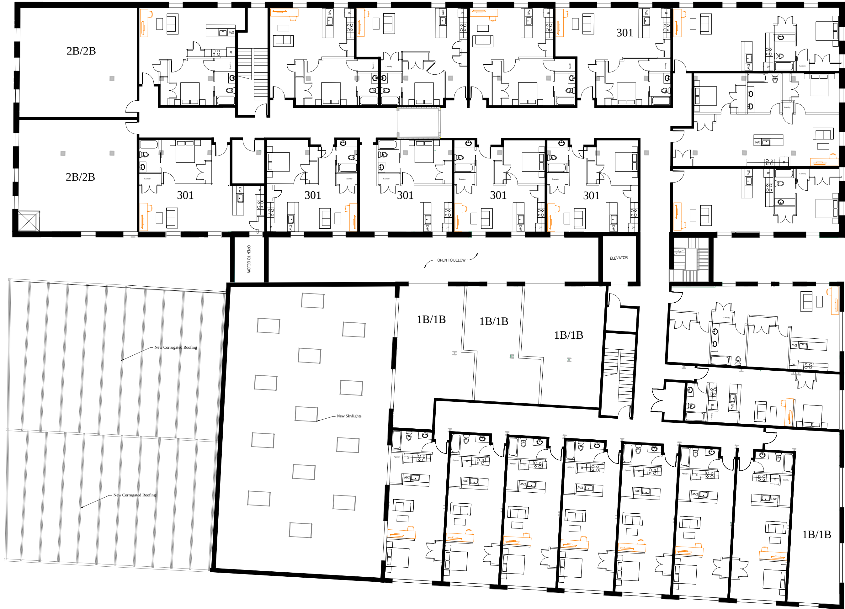
411 Craghead - Existing Conditions & Demo Plan First Floor
