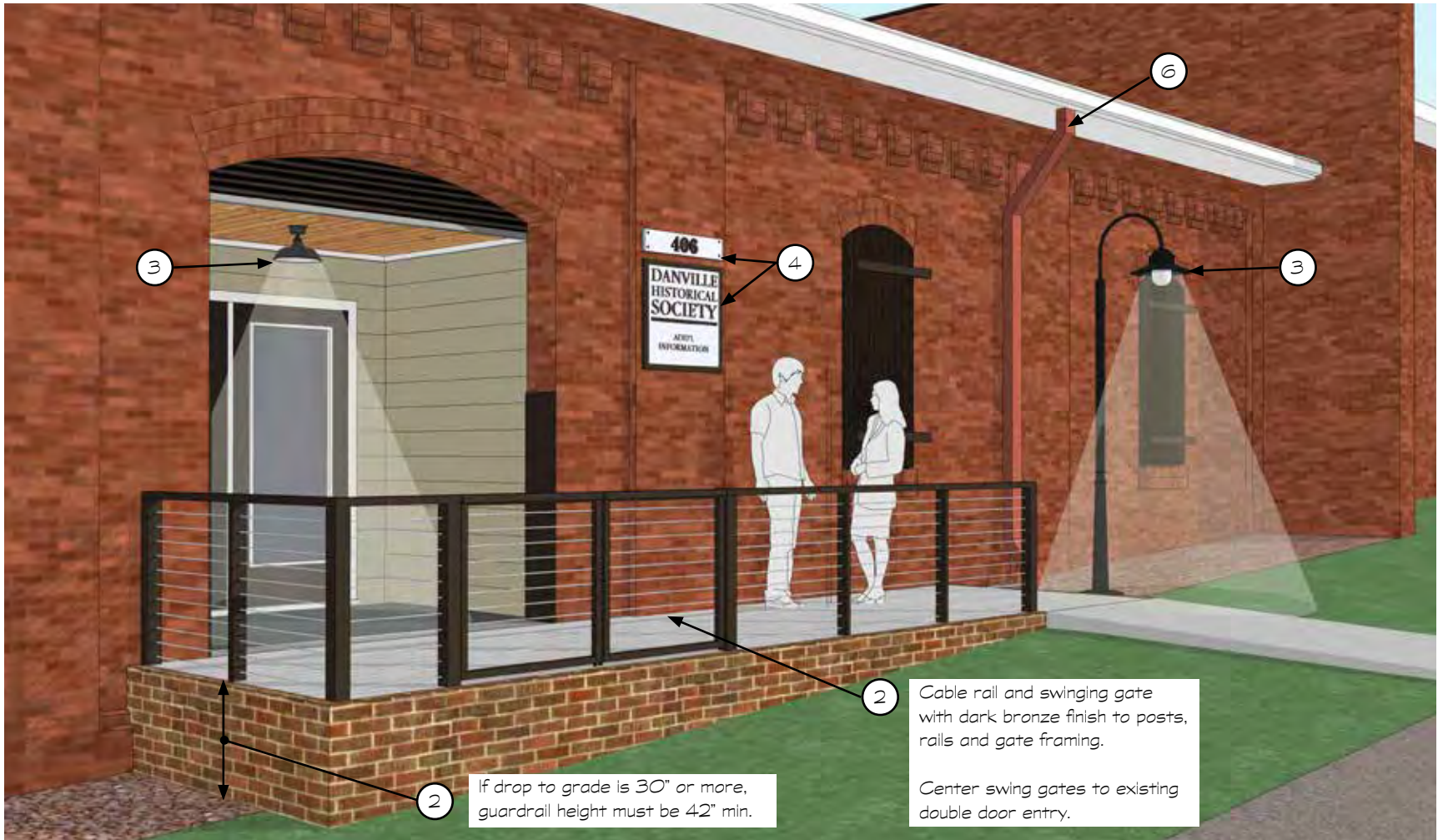
FRONT WALK - OPTION B, CABLE RAIL WITH DARK BRONZE RAILING
