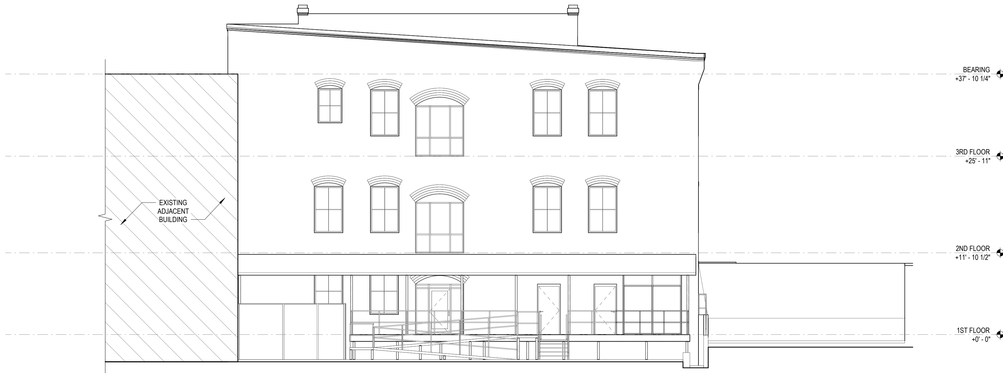
3 A4 1/8" = 1'-0" RENOVATION EXTERIOR ELEVATION
