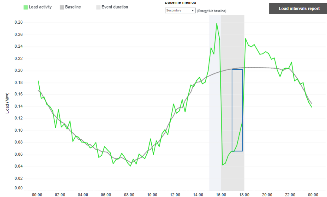
Sample Event: baseline is the gray line; event duration gray block— shows one-hour precool, two-hour event; green line is the AC load. The load shed was 1.23 kW/thermostat during the CP hour (the blue box HE 18), achieved 115.4 kW total load shed for CP hour. The load spike before the event is due to precooling; the load spike after the event is from the AC load coming back online.
